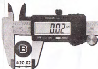
Differential method measurement (Application of zero setting)
