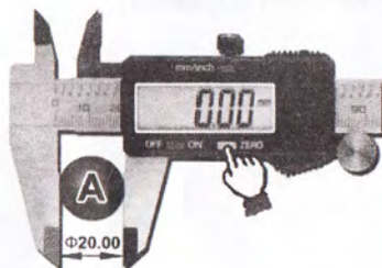
Differential method measurement (Application of zero setting)
